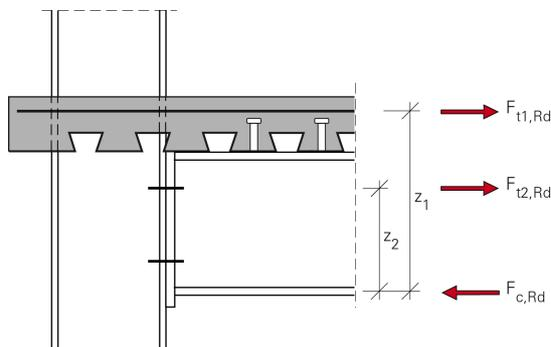
5.25 *Beam-to-column joint with an end-plate.*
