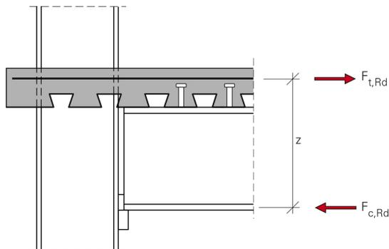
5.24 *Beam-to-column joint with a contact plate.*
