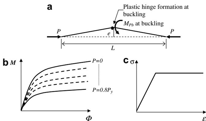
Fig. 2. (a) Nonlinear brace buckling model; (b) moment–curvature relationship of brace cross-section for incremental levels of axial loads to account for moment–axial force interaction; (c) axial stress–strain relationship of the brace.
