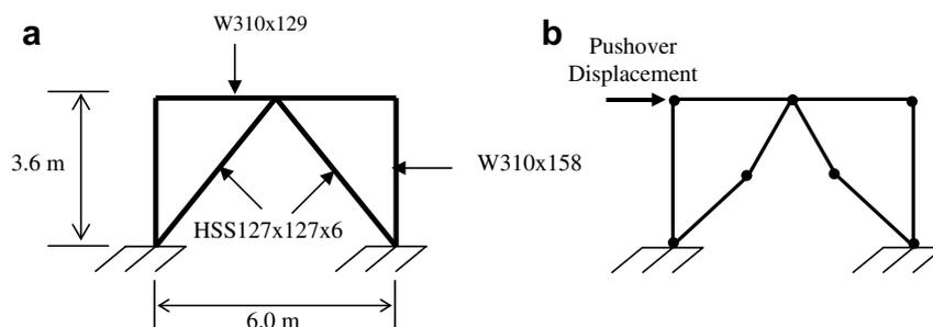
Fig. 6. (a) Single story frame; (b) structural model.
