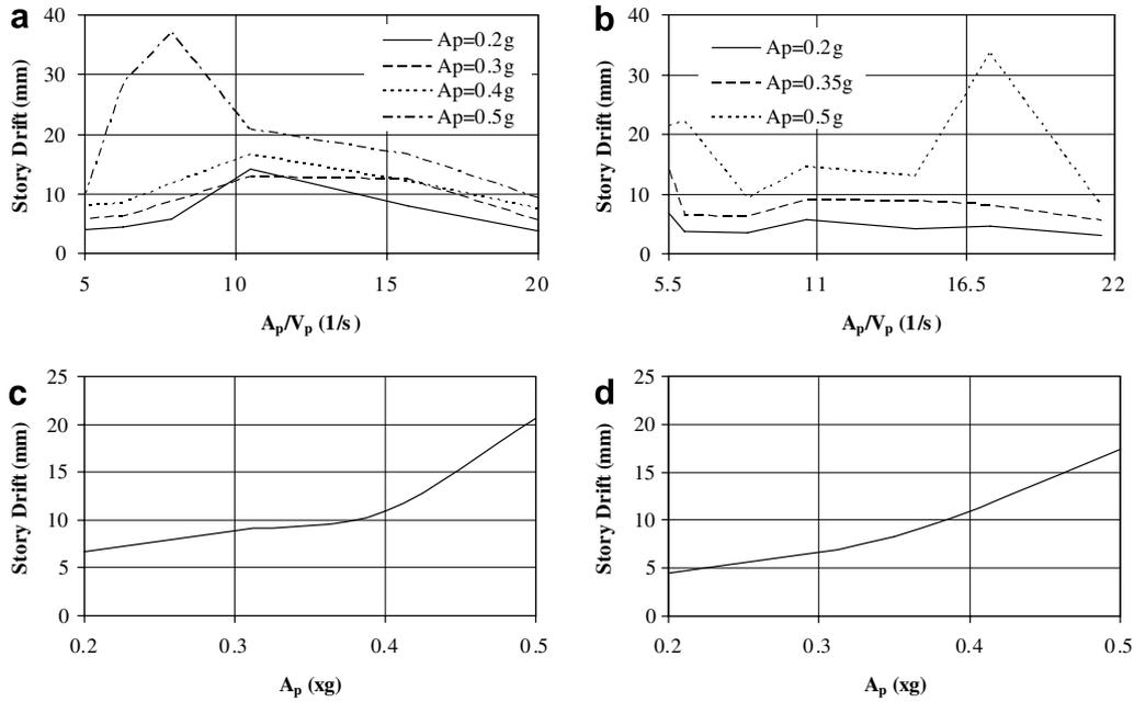
Fig. 9. (a) Story drift vs.  $A_p/V_p$  ratio of harmonic ground motions; (b) story drift vs.  $A_p/V_p$  ratio of seismic ground motions; (c) average story drift vs. intensity of harmonic ground motions; (d) average story drift vs. intensity of seismic ground motions.
