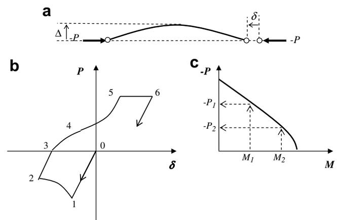
Fig. 1. (a) Displaced shape of steel brace under axial load; (b) typical inelastic cyclic behavior of a steel brace; (c) effect of increased second order moment on axial load capacity.
