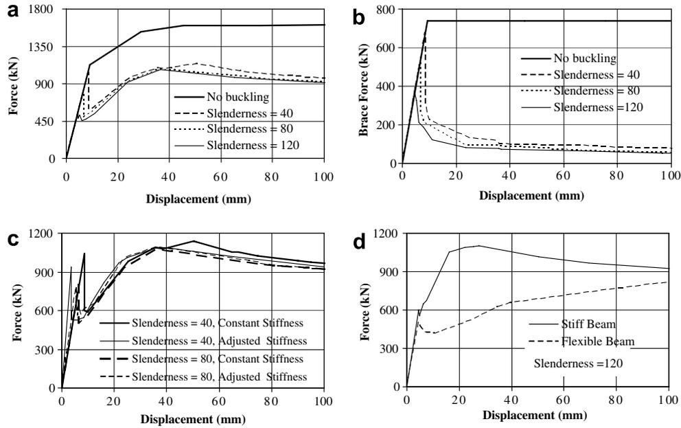
Fig. 7. (a) Lateral force–displacement relationship of frame for various brace slenderness ratios; (b) brace force vs. lateral frame displacement for various brace slenderness ratios; (c) lateral force–displacement relationship of frame for constant and adjusted brace stiffness; (d) lateral force–displacement relationship of frame for stiff and flexible beam.
