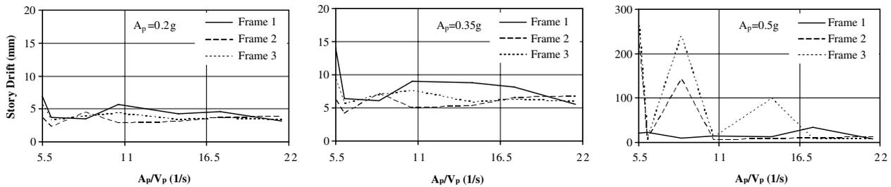
Fig. 10. Comparison of story drifts for CBF with various properties as a function of the  $A_p/V_p$  ratio of seismic ground motions for  $A_p = 0.2$  g, 0.35 g and 0.5 g.
