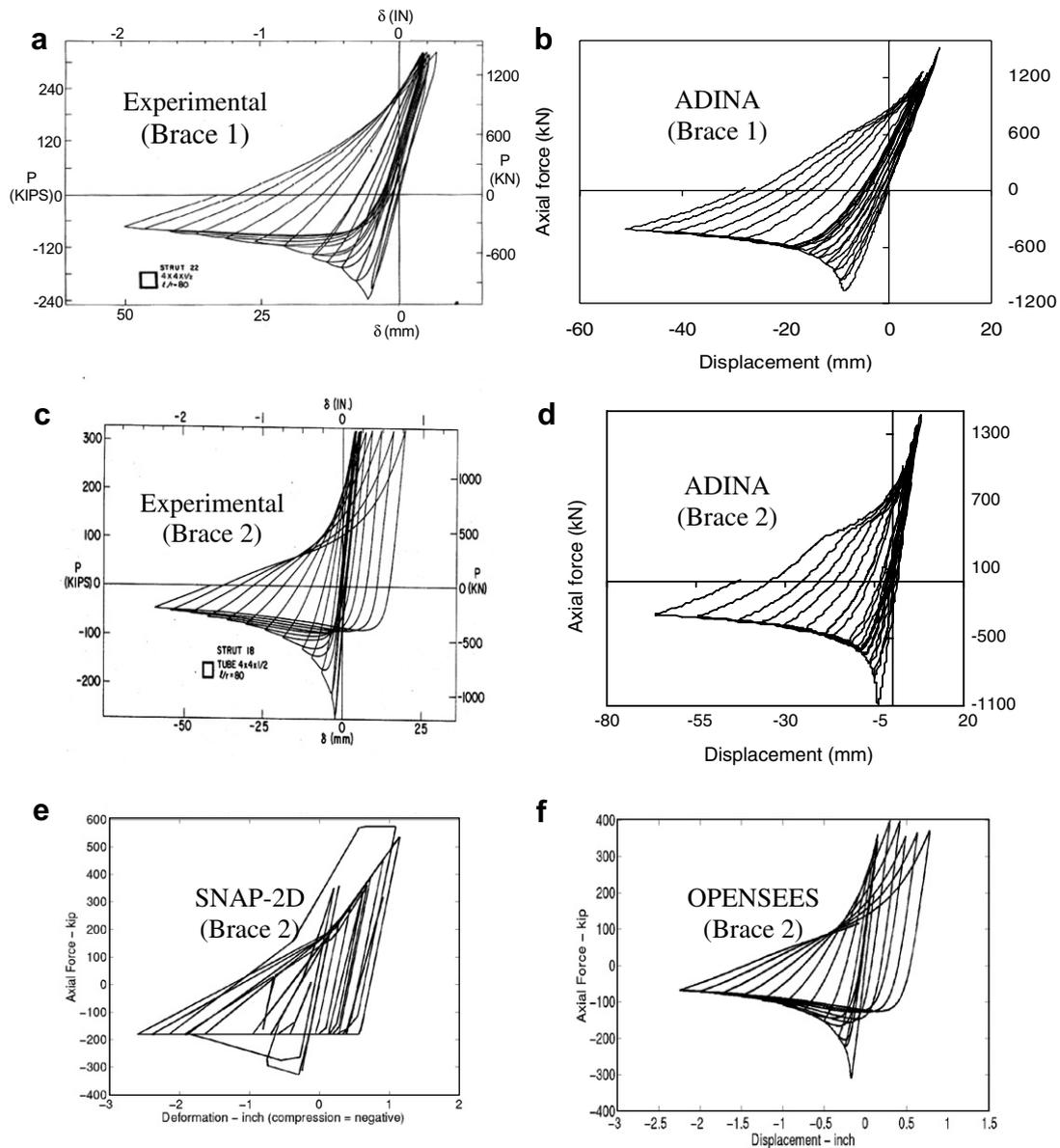
Fig. 5. Comparison of experimental [12] and analytical results for brace specimens: (a) test results for Brace 1; (b) ADINA results for Brace 1; (c) test results for Brace 2; (d) ADINA results for Brace 2; (e) SNAP-2D results for Brace 2 [8]; (f) OPENSEES results for Brace 2 [8].
