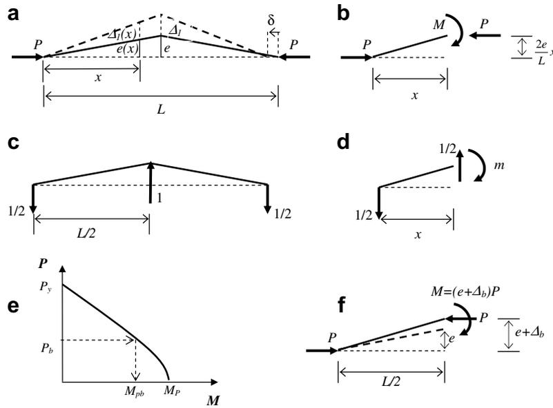
Fig. 3. (a) Effective eccentricity under axial load; (b) free body diagram of the brace to the left of section at  $x$ ; (c) unit dummy load applied at the vertex of the brace element; (d) free body diagram for the unit dummy load; (e) reduced plastic moment at buckling load; (f) second order moment at the vertex of the brace element at buckling.
