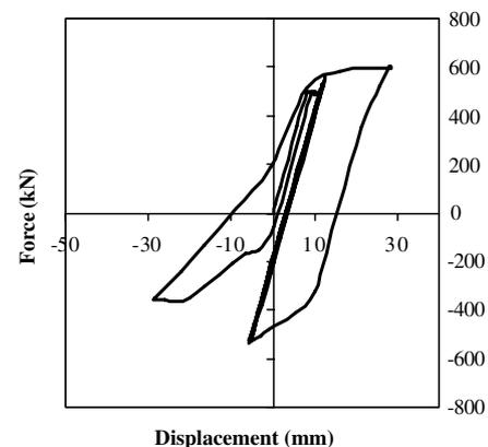
Fig. 8. Force–displacement hysteresis loop of the frame subjected to the harmonic ground motion with  $A_p/V_p = 6.28 \text{ s}^{-1}$  and  $A_p = 0.5 \text{ g}$ .
