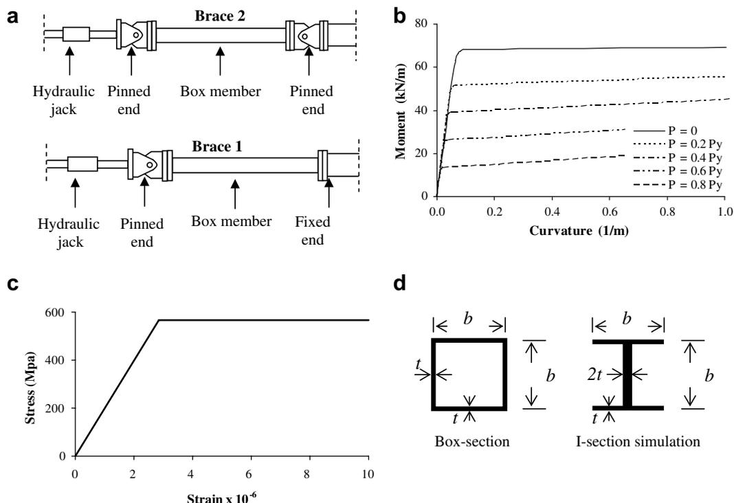
Fig. 4. Properties of box sections used for verification analytical model: (a) details of test specimens [12]; (b) moment–curvature relationships; (c) axial stress–strain relationship; (d) I-section simulation of box-section.
